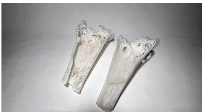
Figure 4 – Printed 3D model. ABS, FDM printing
