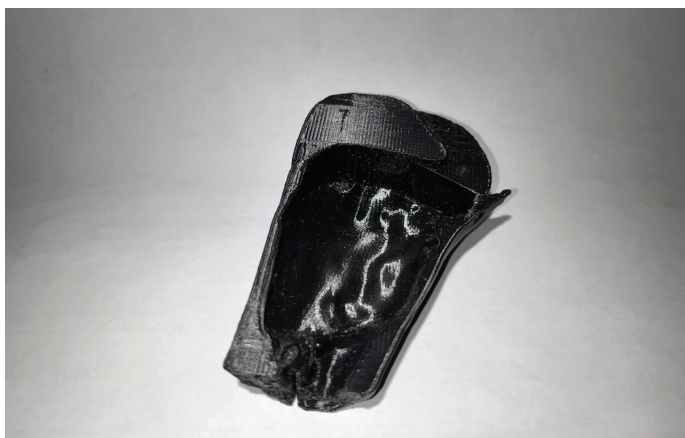
Figure 5 – Printed 3D model. Thermopolyuretan, FDM printing
